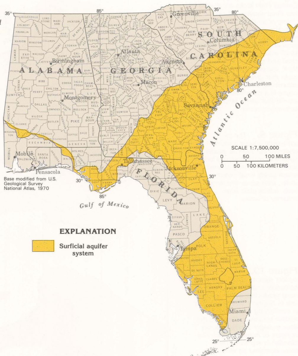
Figure 15. The surficial aquifer system extends throughout large areas in the Coastal Plain of Florida, Georgia, and South Carolina.
