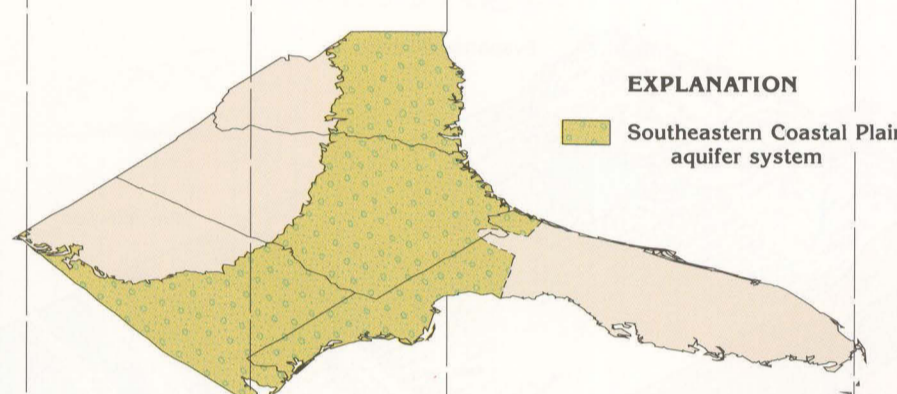
Figure 11. The clastic rocks of the Southeastern Coastal Plain aquifer system yield moderate volumes of water. The clastic rocks underlie the Floridan aquifer system in places, and grade laterally into the Floridan in other places. A clayey confining unit separates the two systems in Alabama and western Georgia.
